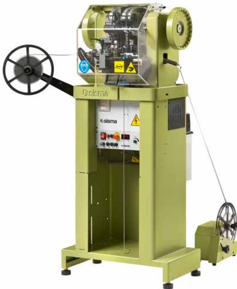
A leading company in the design and manufacture of high-precision chain machines, Sisma presents a new evolution of its SSK, a version that not only produces real "Snake" chain in its round version, but also in oval and elongated, flattened versions, known as "Sole".
